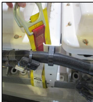
Figure 35: Safety Hook Attached to ESS Rooftop Rail
