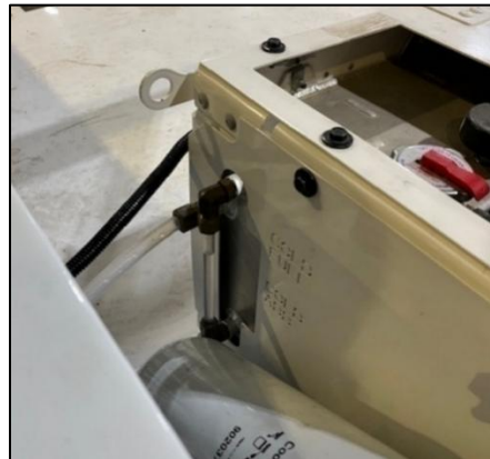
Figure 42: BTMS Sight Glass
