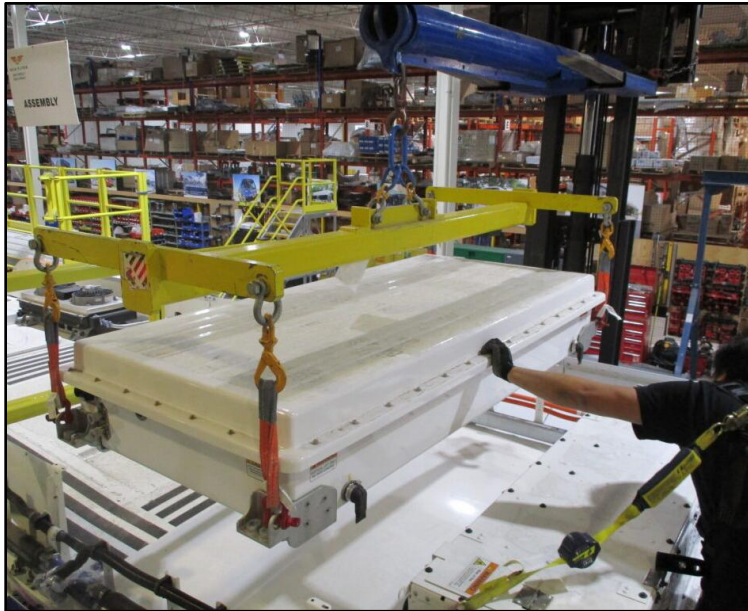
Figure 36: Lifting the ESS from Rooftop
