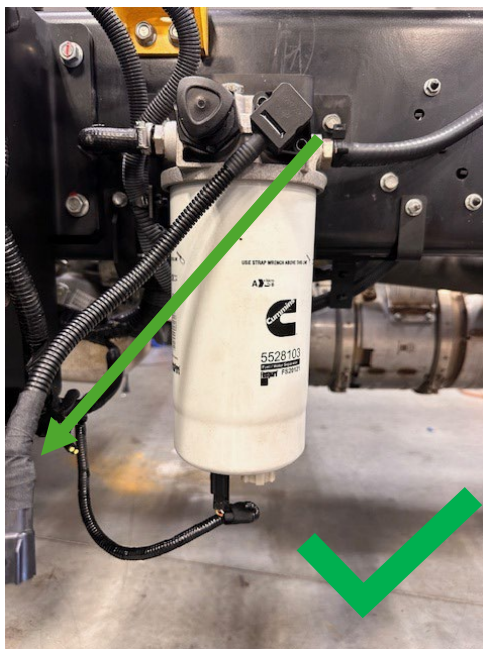
Figure 6 – Correctly Installed Fuel Heater
