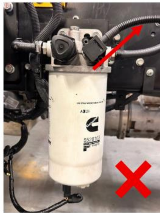
Figure 7 – Incorrectly Installed Fuel Heater
