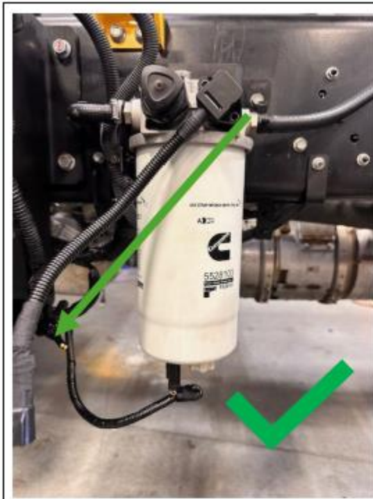
Figure 6 – Correctly Installed Fuel Heater
