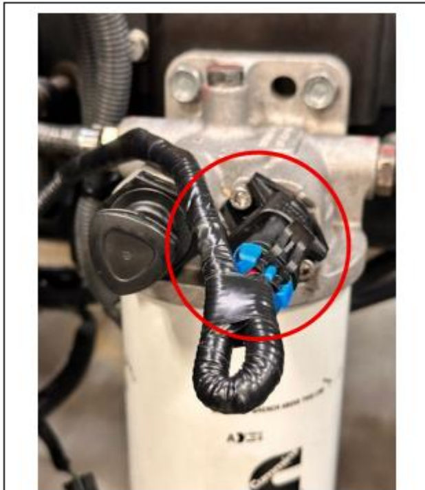
Figure 2 – Fuel Heater Connector J-303
