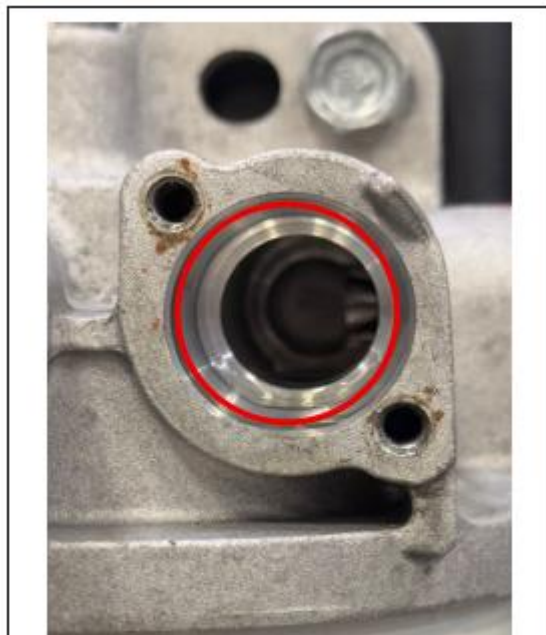
Figure 5 – Clean the Mating Surface Circled in Red
