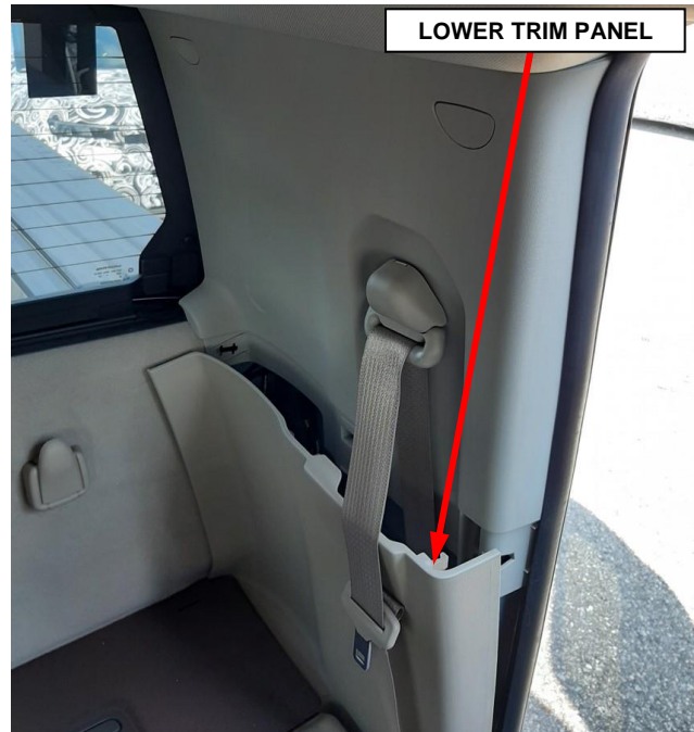
Figure 28 – C-Pillar Lower Trim Panel
