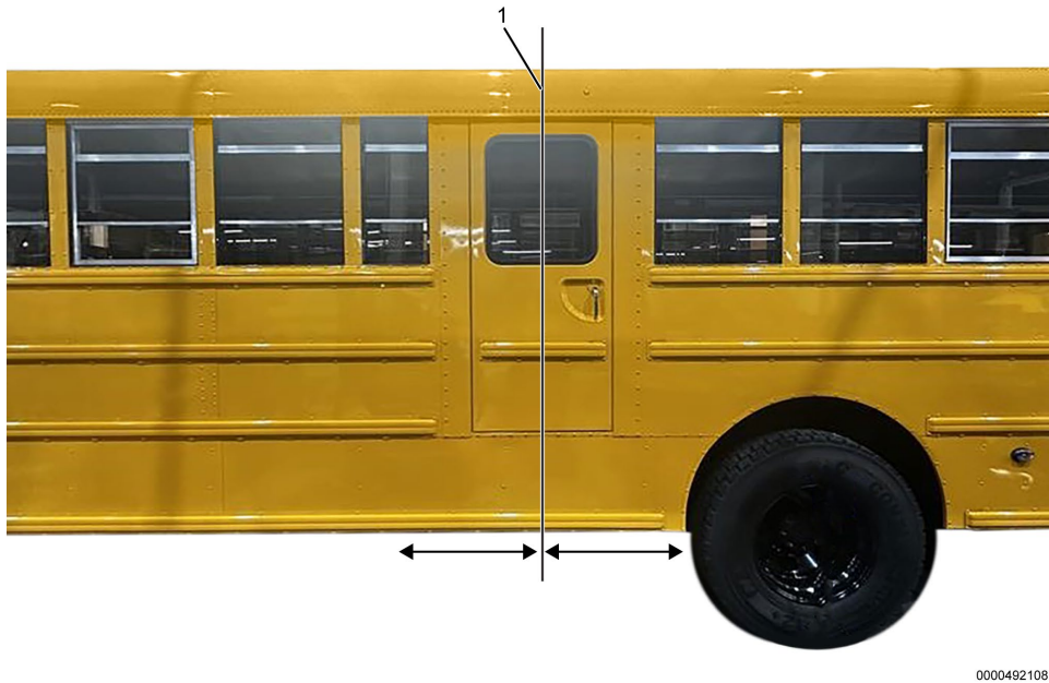
Figure 1. Non-Luggage Compartment Emergency Door 1. Centerline
