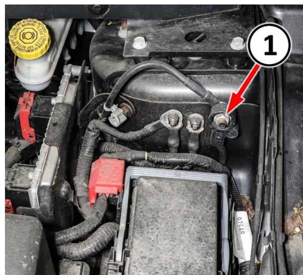
Figure 1 – Battery Negative Cable
