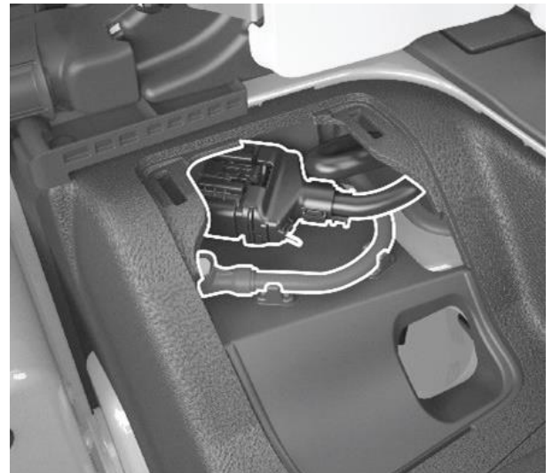
Figure 6 – Wire Harness and Hose Connection Storage Compartment
