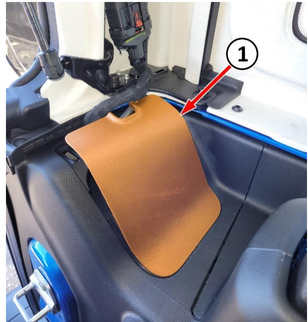
Figure 4 – Storage Compartment Cover
