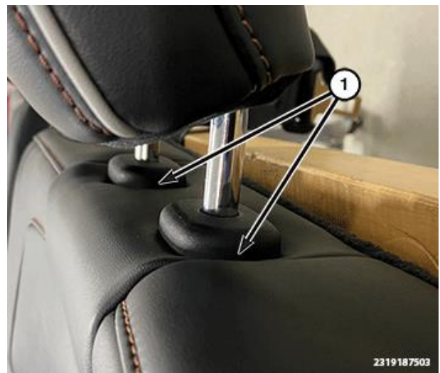
Figure 6 – Early Design Outer Headrest Retainers
