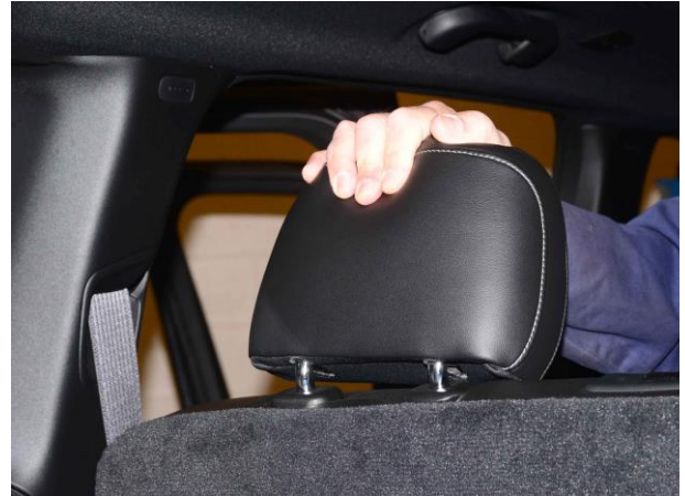
Figure 5 – Testing Headrest – Fore / Aft Motion
