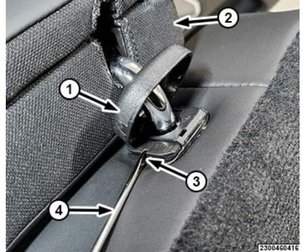
Figure 7 – Late Design Outer Headrest Retainers
