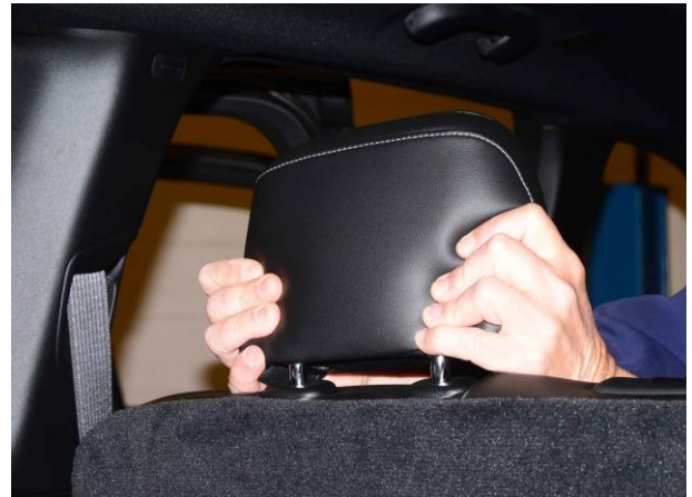
Figure 4 – Testing Headrest – Side to Side Motion
