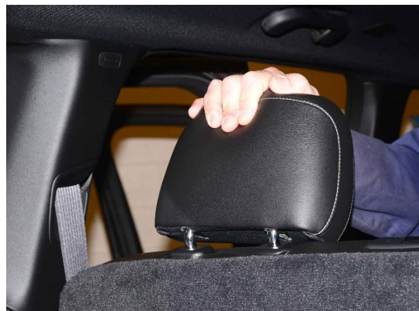
Figure 5 – Testing Headrest – Fore / Aft Motion
