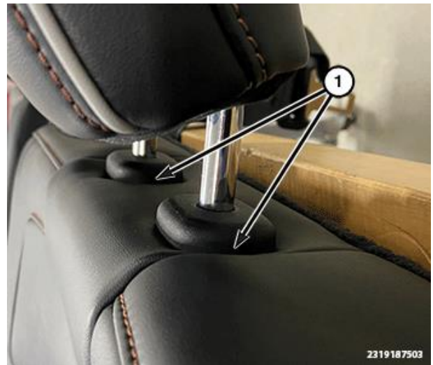
Figure 6 – Early Design Outer Headrest Retainers
