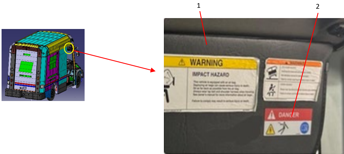
Figure 2. EV Danger Label Removal.
