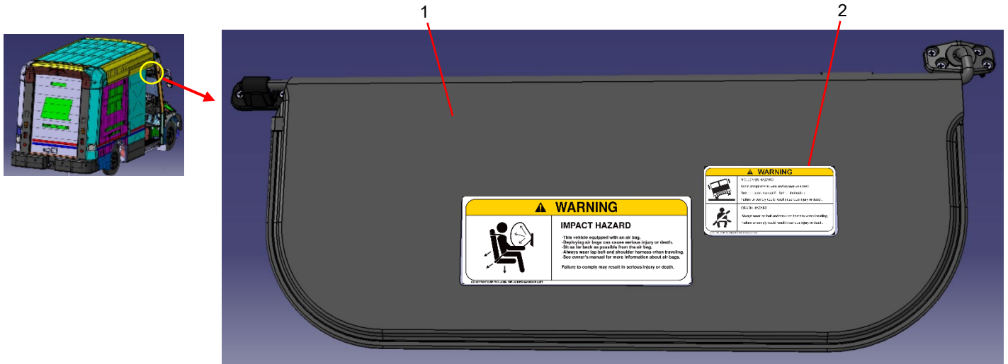
Figure 2. Rollover Warning Label Removal.
