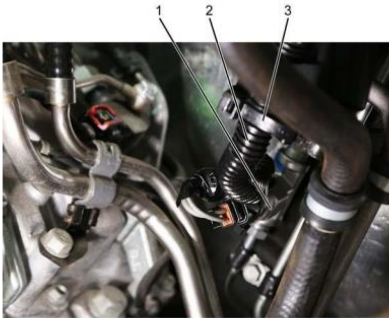
Figure 2. Brake Pressure Switch Connector Location
