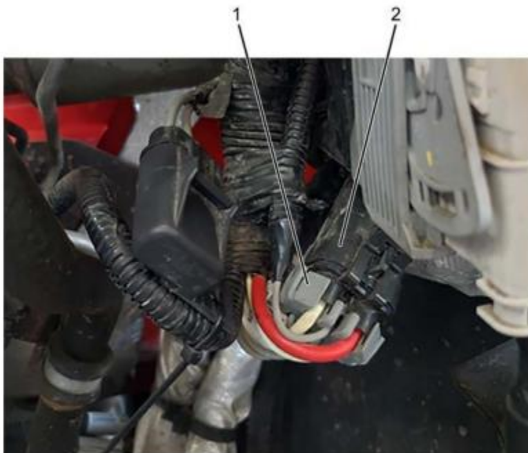
Figure 3. Booster Pump Motor Jumper Harness Connector
