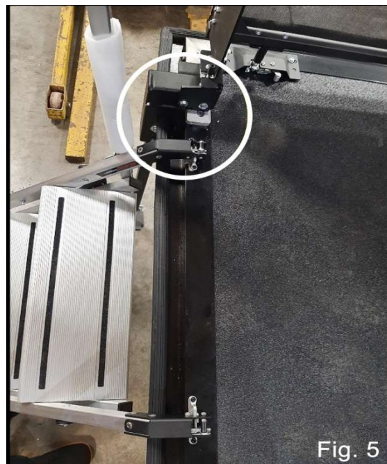
Fig. 5 shows the drop leg keeper assembly with the patio rail drop leg installed, from above.
