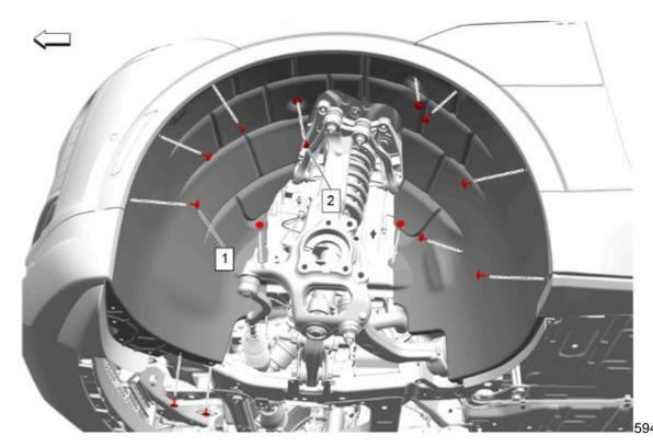
Remove the fasteners from the rear half of the Left Front Wheelhouse Liner and reposition out of the way.
