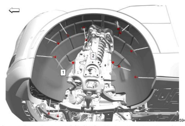
3. Remove the fasteners from the rear half of the Right Front Wheelhouse Liner and reposition out of the way.
