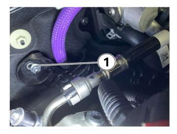
Remove nut from firewall and feed the 48V B+cable out from under the vehicle (cable is disconnected from SGR). (Tighten nut to 9 Nm during assembly)
