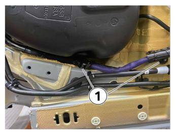
Continue removing plastic nuts and feed out cable (1).
