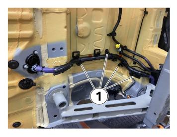
Remove all plastic nuts (and feed the cable out of the trunk. (replace all plastic nuts during assembly and torque to 2.3 Nm)
