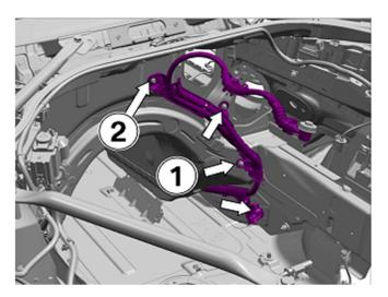
**G45:** There are three plastic nuts (1) (see previous photo) and one metal nut (2) (next step photo) that need to be removed.
