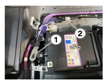
Disconnect the 48V SGR cable (1) from the B+terminal of the 48V battery.
