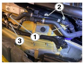
Disconnect low temperature coolant circuit's coolant hose (1) from both ends and remove coolant pipe with bracket (2). (Replace the plastic nuts during assembly and tighten to 2.3 Nm).
