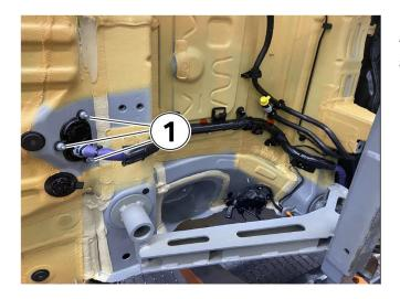
Remove the nuts (1) holding the SGR B+ cable to the trunk. (Replace nuts during reassembly and tighten to 9 Nm)
