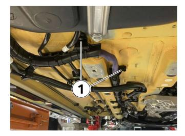
Continue removing plastic nuts and feed out cable (1).
