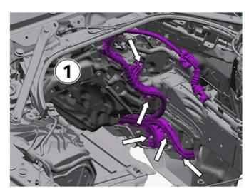
**G60:** Layout of cable in the engine compartment
