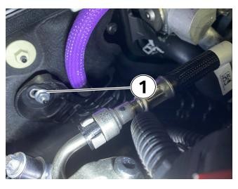
Remove the nut from the firewall and feed the 48V B+ cable out from under the vehicle (cable is disconnected from SGR).
