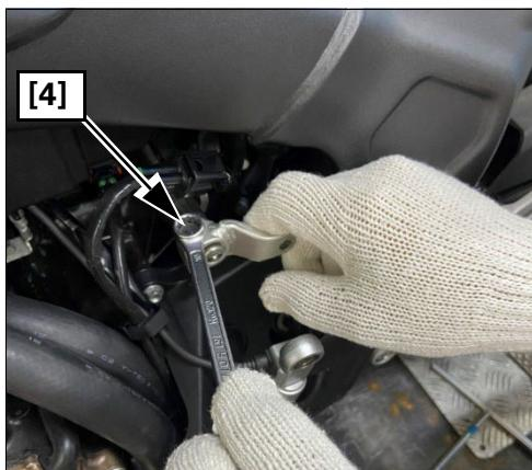
3. Remove the original gearshift arm by pulling it away from the shift shaft. Place the original gearshift arm aside and be sure not to confuse it with the new gearshift arm.
