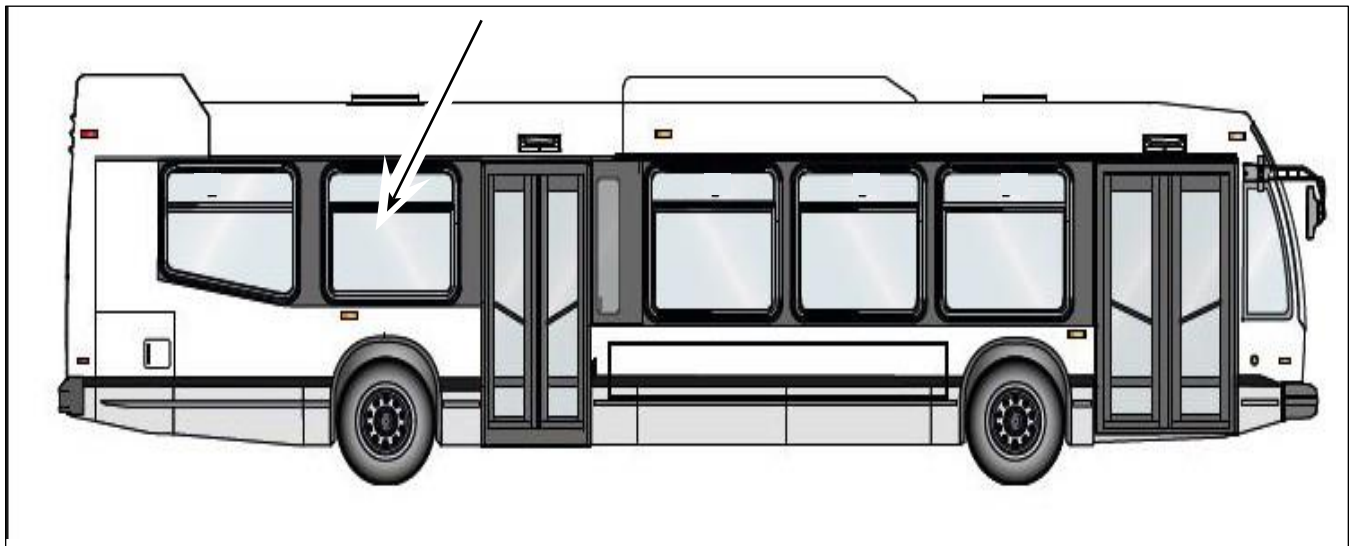
Figure 12 - Location of the Second Window to Replace by N93837-82
