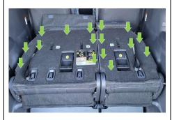
c. Align back board and push to secure all clips.
