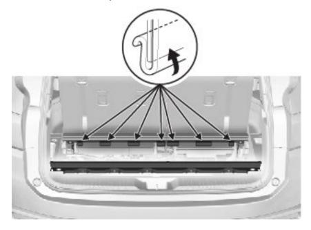
8. Remove the two bolts and seat bar.
