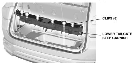
6. Pull on the forward garnish to release the clips and tabs, then remove the forward garnish.
