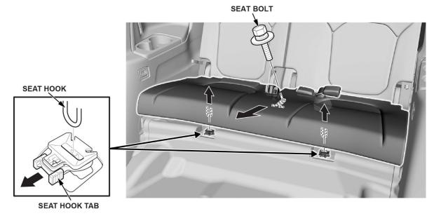
11. Remove the harness clips and disconnect the harness connector, then remove the four mounting bolts from the 3<sup>rd</sup> row right passenger seat only and remove the seat.
