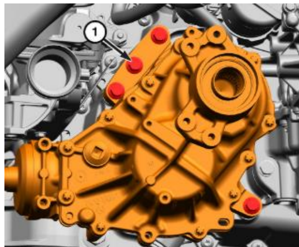
Figure 25 – PTU to Transmission Bolts
