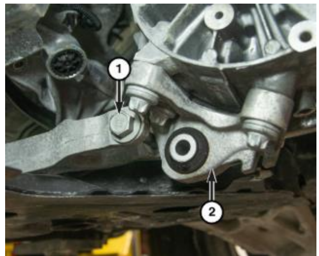
Figure 7 – Rear Engine Mount Bracket and Isolator
