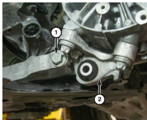
Figure 29 – Transmission Pivot Bracket
