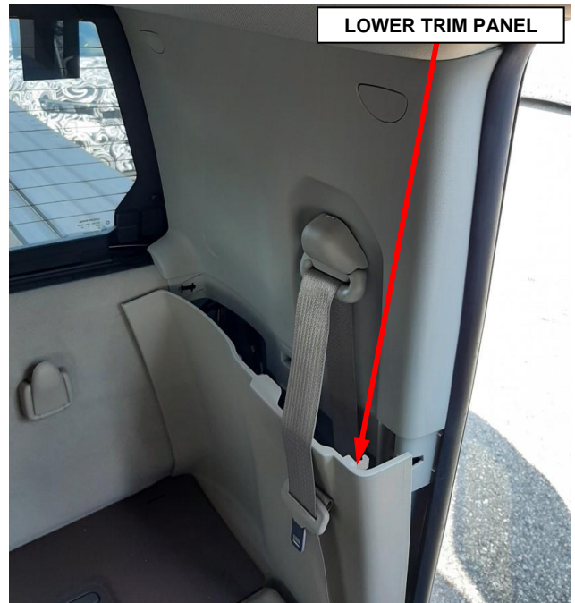
Figure 28 – C-Pillar Lower Trim Panel
