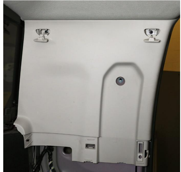
Figure 30 – C-Pillar Upper Trim Panel Fasteners
