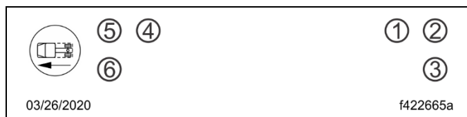
Fig. 4, Tightening Pattern, Right-Front Bendix Axial Caliper
