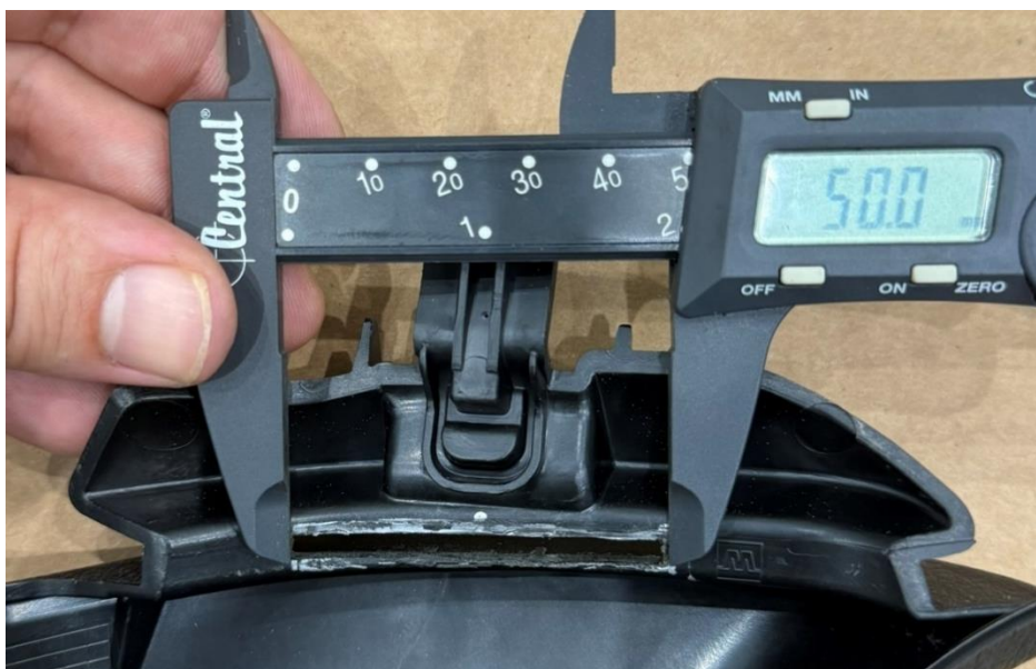
Figure 8 (Right C-pillar trim, back side after cutting and removing residual material debris)
