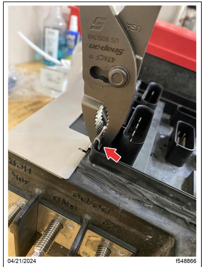
Fig. 8, Bending Over the Bracket Tab with Pliers
