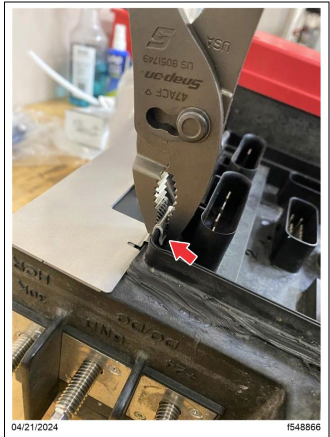
Fig. 7, Bending Over the Bracket Tab with Pliers
