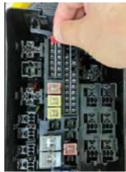
3 rd Remove and insert the fuse five times
