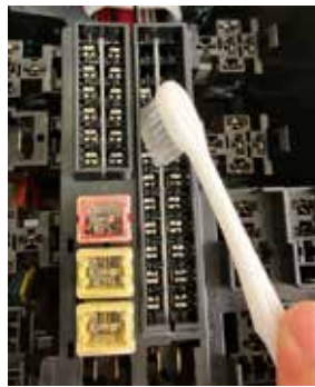
2 nd Clean the fuse terminals with a brush
