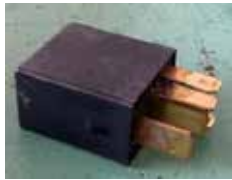
The outside surface of relay terminals have rusted
