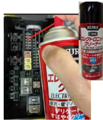
4 th Apply electronic cleaner like KURE 3012 or TUNAP375 or its equivalent
