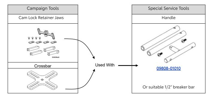
Camry uses a cam-lock type retainer as shown below.
