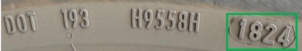
Figure 1 – example of DOT date code
