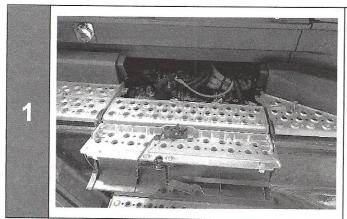
Locate the 200A APU battery cable fuse holder in the truck battery box.
