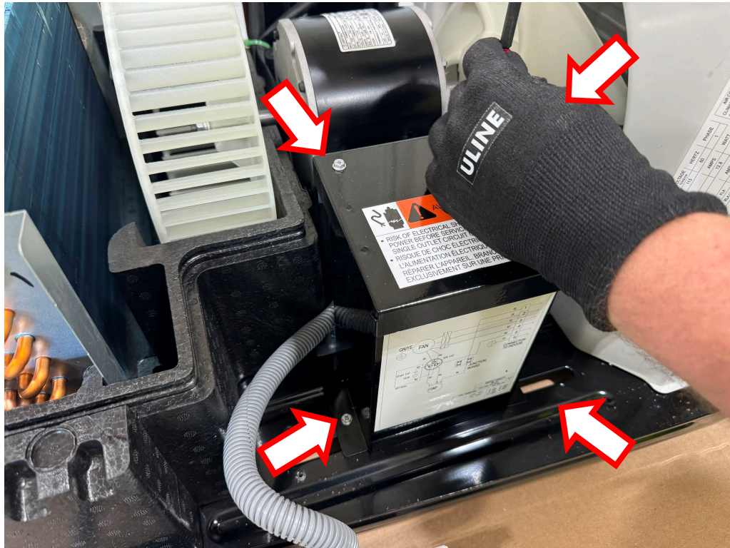
Step 1: Remove 4 Phillips-head screws
