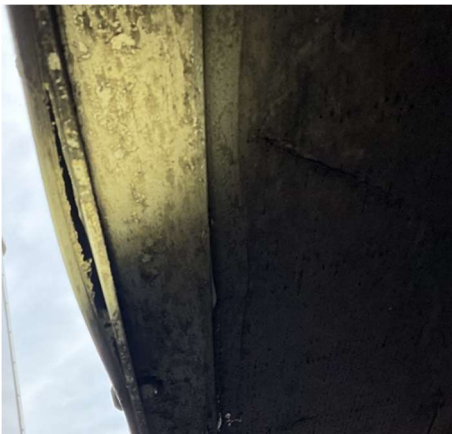
Figure 7: Baserail bulging at bottom. View from underneath trailer.
