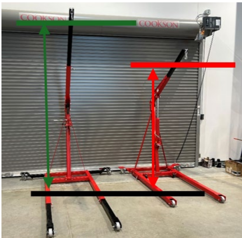
Engine Hoist Height Comparison (Hoist on left is Recall SST, hoist on right is normal hoist offered through ADE Program)
