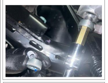
Photo #4 of completed steering gear housing with the black cover. Note the added silicone sealant is on the end cap nut. <u>Note</u> paperless dealers or to save printing costs do not have to have the RO in frame just the written RO# on the steering rack.
