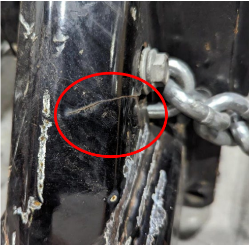
Photo 2 Example of crack near safety chain location
