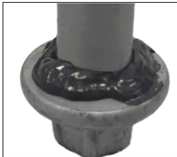
TYPICAL – APPLY LOCTITE 5910 UNDER SCREW HEAD
