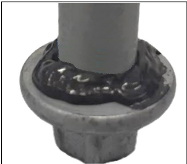
TYPICAL – APPLY LOCTITE 5910 UNDER SCREW HEAD
