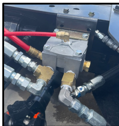
Figure 3.2 Correct Valve on the Right Side
