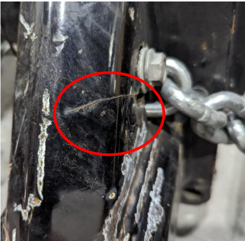
Photo 2 Example of crack near safety chain location
