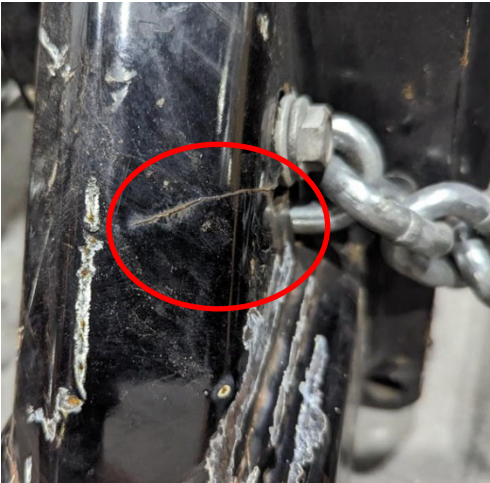
Photo 2 Example of crack near safety chain location
