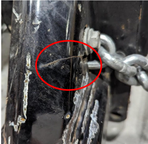
Photo 2 Example of crack near safety chain location
