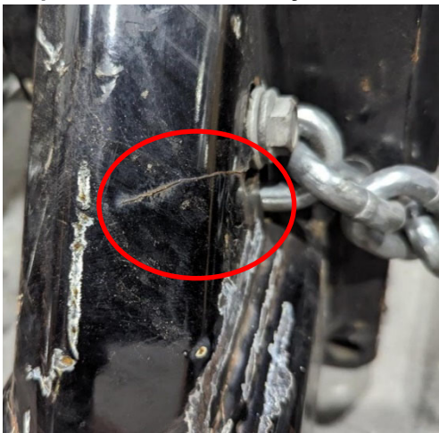
Photo 2 Example of crack near safety chain location
