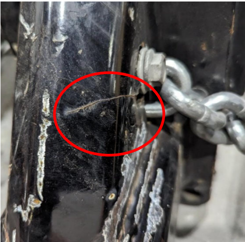
Photo 2 Example of crack near safety chain location
