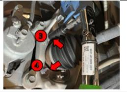
e. Loosen then torque the passenger side hub bolts (3) and (4) to specification.
