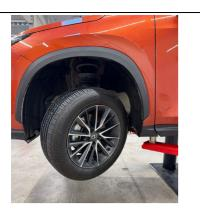
d. Turn the driver front wheel full mast to the left (towards driver side).
