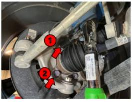
c. Loosen then torque the driver side hub bolts (1) and (2) to specification.
