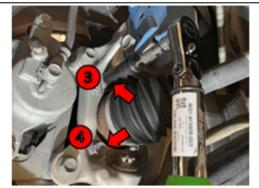
e. Loosen then torque the passenger side hub bolts (3) and (4) to specification.
