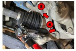
e. Loosen then torque the driver side hub bolts (3) and (4) to specification.
