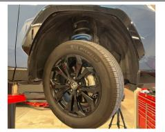
d. Turn the driver front wheel full mast to the right (towards passenger side).
