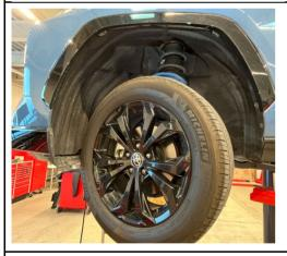
c. Turn the driver front wheel full mast to the right (towards passenger side).
