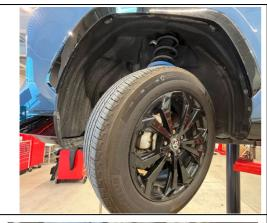
d. Turn the driver front wheel full mast to the left (towards driver side).
