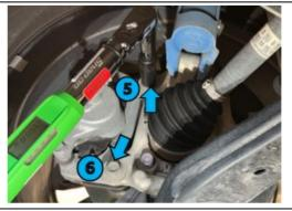
f. Loosen then torque the passenger side caliper bolts (5) and (6) to specification.
