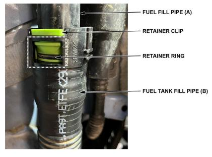
3. Verify the fuel tank fill pipe (B) is firmly connected by pulling down on the lower portion of the tank fill pipe.
