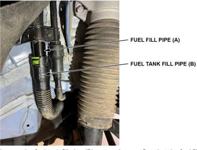
2. Inspect the fuel tank fill pipe (B) connection, confirm that the fuel fill pipe (A) retainer ring is visible in the retainer clip window.
