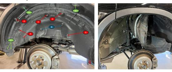
1. Use compressed air and a clean shop towel to clean around the fuel fill pipe (A) and fuel tank fill pipe (B).
