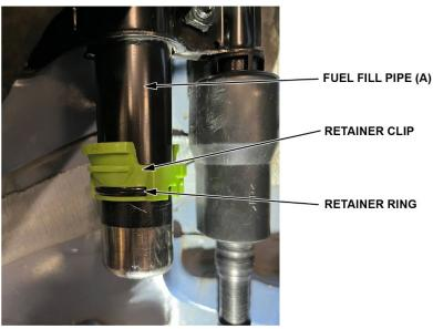
4. Install the fuel tank fill pipe by sliding the pipe onto fuel fill pipe and retainer clip. Make sure the fuel tank fill pipe clicks onto the retainer clip.
