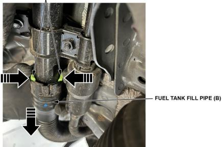
2. Use a clean shop towel to clean the outside areas of the fuel tank fill pipe and fuel fill pipe.
