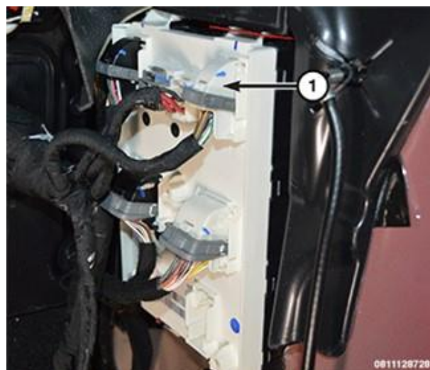
Figure 50 – Body Control Module (BCM) 1 - Wire Harness Connector
