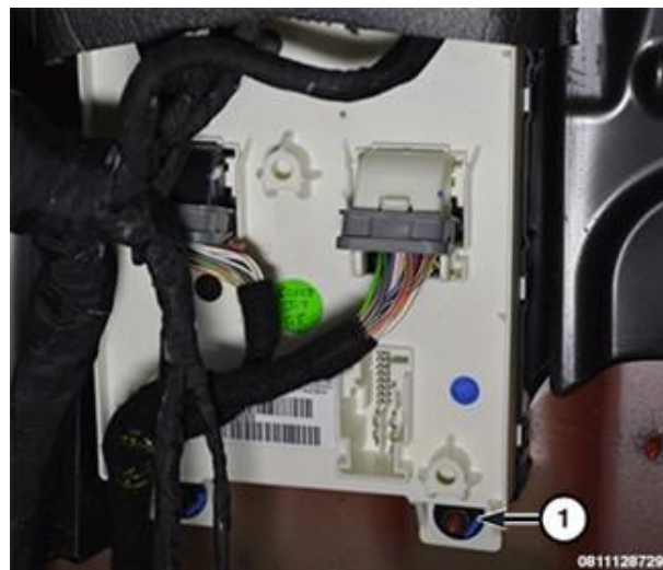
Figure 49 – Body Control Module (BCM) 1 - Mounting Bracket Fastener
