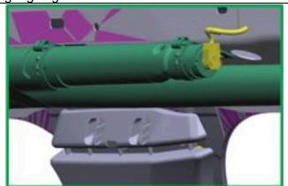
The head air bag right gas generator electrical connector (shown here in yellow) is oriented towards the roof of the vehicle.
