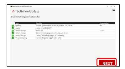
(5) When the software is being updated and advances to 90% on the screen, it may stop advancing for about 60 seconds. Wait until reprogramming is complete.
