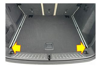
Remove and replace each of the rear screws (arrows) that secure the left and right cargo rails with a new screw. The washers can be reused.
